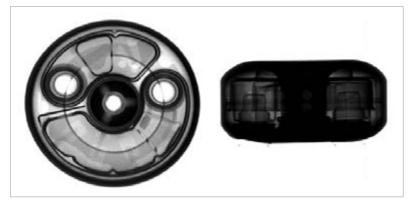
Driver-side airbag containing the igniter system
