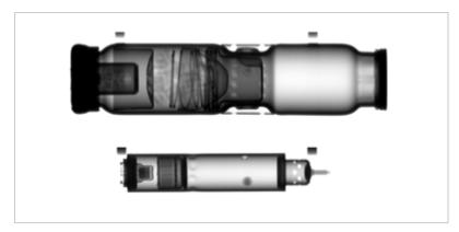
Passenger and side-impact airbag containing the igniter system
