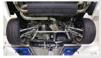
The undercarriage of an automobile showing metal struts connecting to the suspension system near each wheel
