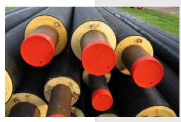
Sections of insulated heat pipe with embedded sensors
