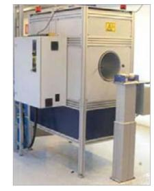
X-ray cabinet system for testing pre-insulated heat pipe systems during production
